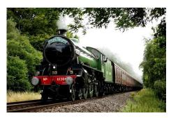
Built for the London & North Eastern Railway, 61306 Mayflower is one of two surviving B1 Class locomotives. The B1's were designed as mixed traffic locomotives capable of hauling express passenger trains as well as freight traffic. As powerful, go anywhere engines, the B1's worked across most of the UK rail network from East Anglia to Scotland.
